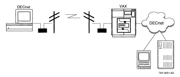
Figure 1–3 shows a typical asynchronous configuration. This configuration uses a telephone line between a Macintosh computer that runs DECnet software and a VAX computer that is a DECnet router. 2400 baud modems and RS-232C cables connect the computers to the telephone line.
